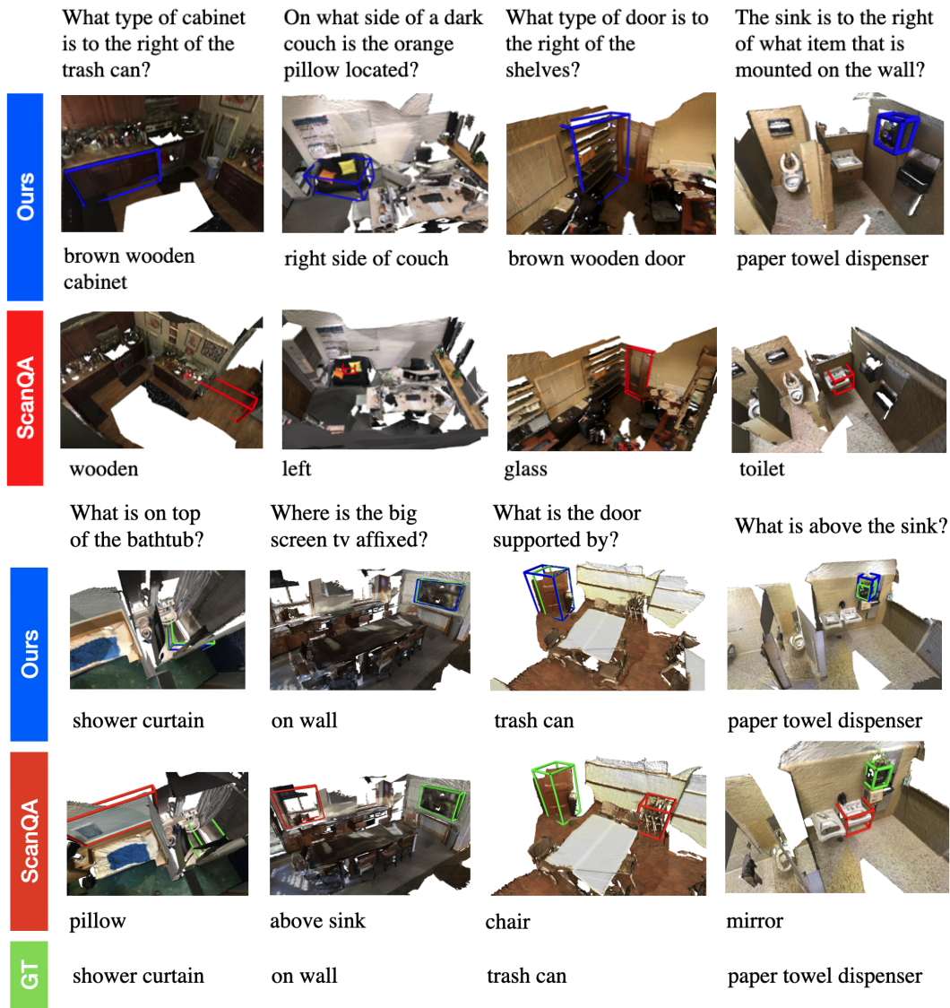
Figure 3. Example questions and answers from the test set with object IDs (top) and the validation set (bottom). We compare the results of our model (blue) to ScanQA [4] (red) and the ground truth (GT) (green). Below every image is the predicted or generated answer. Since we do not axis-align our scenes, the bounding boxes in our model look tilted. We include more examples in the appendix. Best viewed in color.
